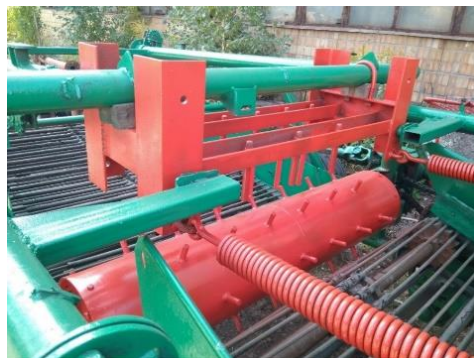
Fig. 4. Grinding apparatus of the machine for separating miscanthus rhizomes into parts and rhizomes
